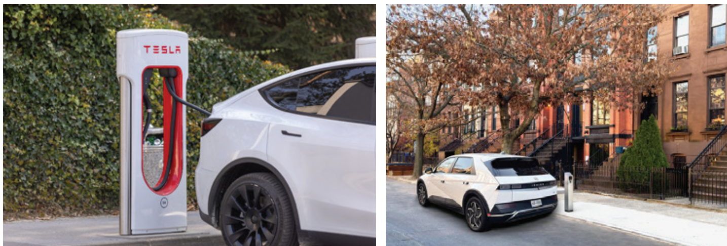
Figure 4. Two approaches to EV charging: Left: The Tesla network of Level 3 fast charging stations can deliver 100 miles of range in 10 minutes, ideal for highway settings. Right: Community curbside charging, such as this prototype Level 2 charger from Itselectric, delivers the same range in about 4 hours, and is more suited to workplace and home.
