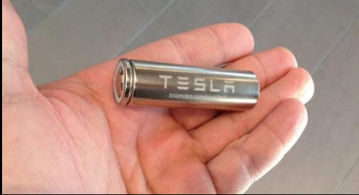
Tesla nominal cell voltage: 3.6 Volts
