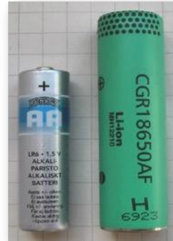
18650 cell format used in 85 kWh Tesla battery
